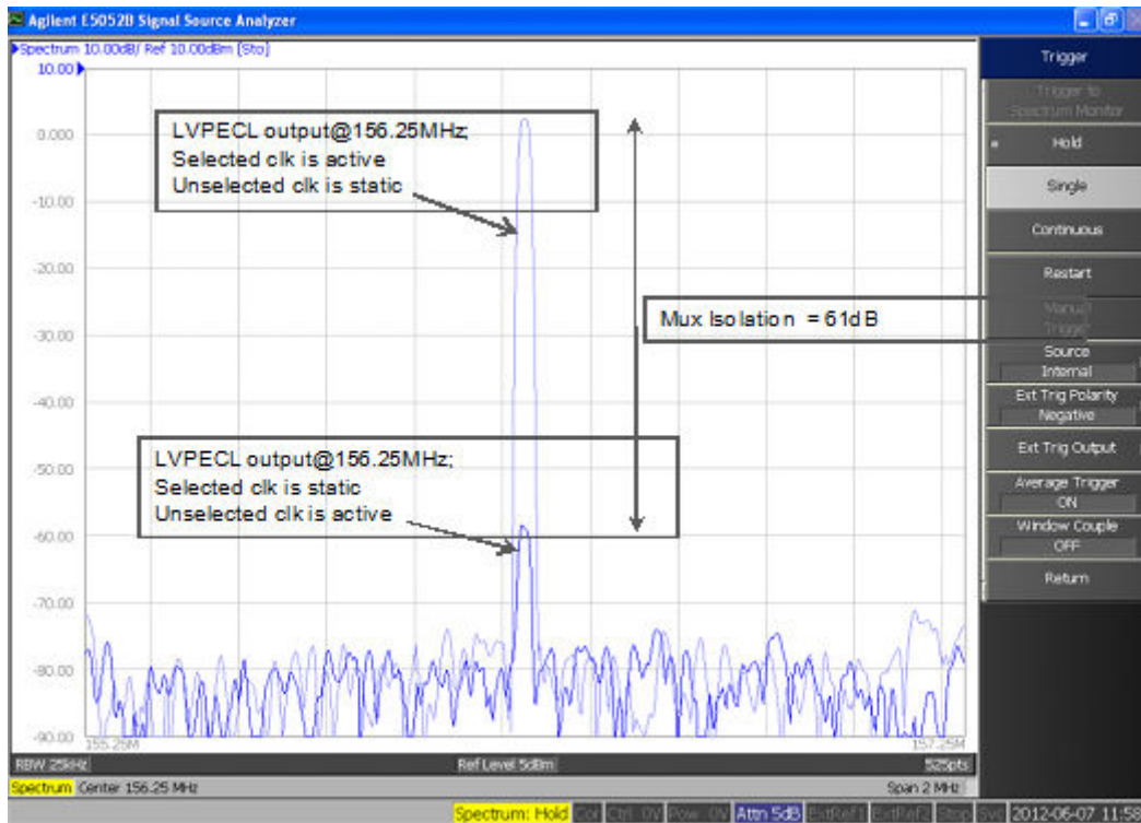
Figure 2.13. Input Mux Noise Isolation (Differential Input Clock, 44-QFN Package)
