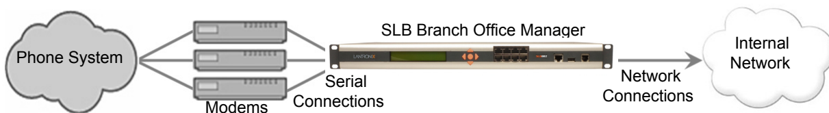
Figure 10-2 Remote Access Server
