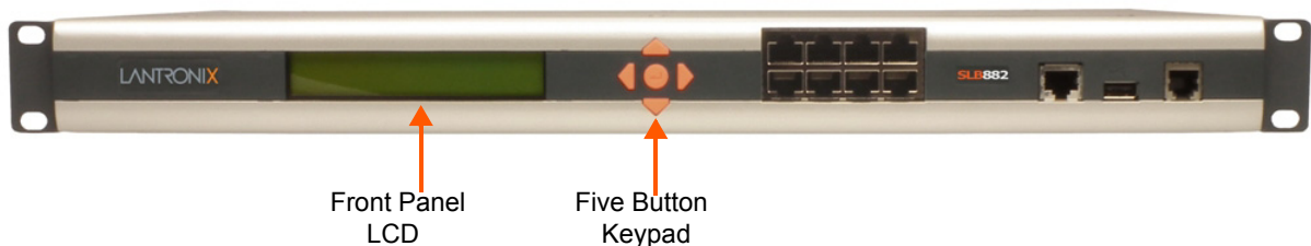
Figure 4-2 Front Panel LCD Display and Five Button Keypads (Enter, Up, Down, Left, Right)
