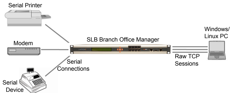
Figure 10-4 Multiport Device Server
