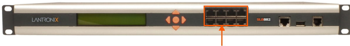
Figure 2-6 Device Port Connections
