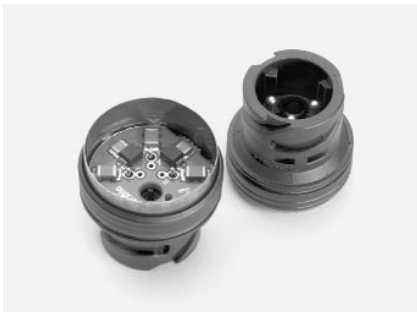
Pressure transmitter sensor-connector with PCB terminals. (Other termination methods are possible). Connector is fixed either by flared joint or over-mold.
