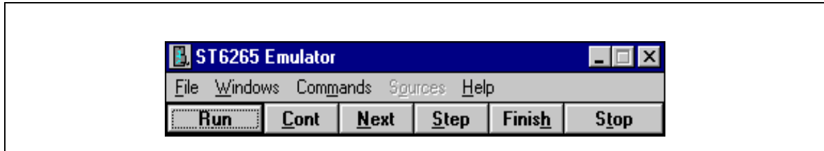
Figure 9: Control Bar window
