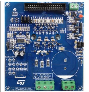
Figure 1: Motor control board (top view) based on SLLIMM-nano<sup>™</sup> 2nd series
