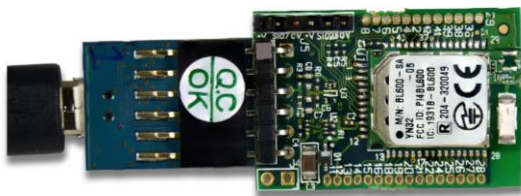
Figure 19: BA600-0x connected to the USB-UART bridge board
