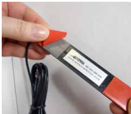
Adhesive Mount Antenna – Step 2. Peel Protection from Adhesive Strip
