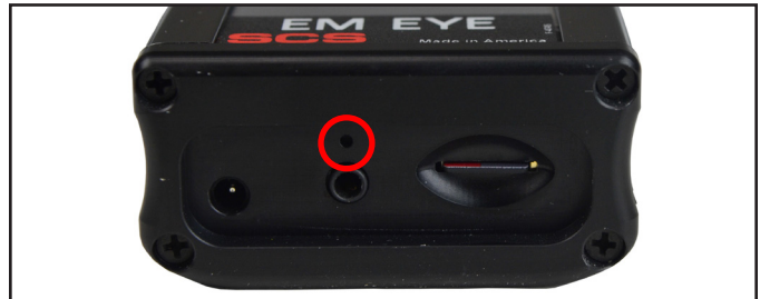
Figure 7. Location of the reset button at the bottom of the EM Eye Meter
